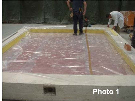
Photo 1: Position of “Sylomer” in the perimeter and film of PVC on normalized heavyweight floor
