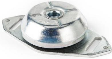
AMC Mecanocaucho® BRT anti vibration mounts are anti vibration elements which work the rubber in shear and compression with an optimal ratio of stiffness and horizontal stability. These engine mounts are really applicable as stabilizers of electrical cabinets or racks. Thanks to the robust fail safe architecture it is useful In applications where the box type assembly is submitted to shocks.
